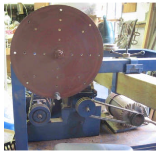
Opposite side of lathe showing mounting plate for compensating weights
