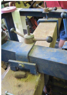
Mounting of wood beam part of tool rest system
