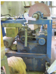
Turning side of lathe showing tool rest supported by wood beam
