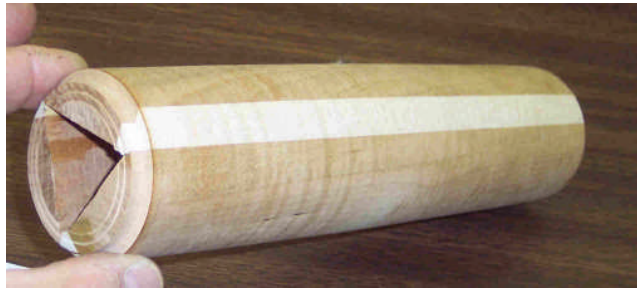
Kaleidoscope barrel with space for the insertion of the three mirrors
