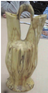
Bernie -a hollowform native American wedding vessel made of Spalted Birch, hollowed thru the bottom, plugged, then turned each spout from a different center on the base (turn one, finish then remove a section of the base leaving a second section to hold piece for turning the other spout).
