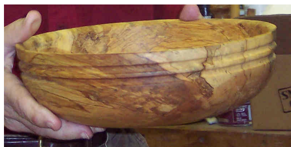
Sid Katz -a spalted Maple bowl. It was punky wood so he poured CA glue over it & it hardened up enough to turn. Finished with Mahoney's walnut oil.
