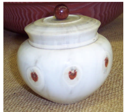
This is a Norfolk Island Pine box by Jeff who turned it, bleached it several times with two part wood bleach, neutralized it with vinegar and finished it with Minwax waterbase varnish.
