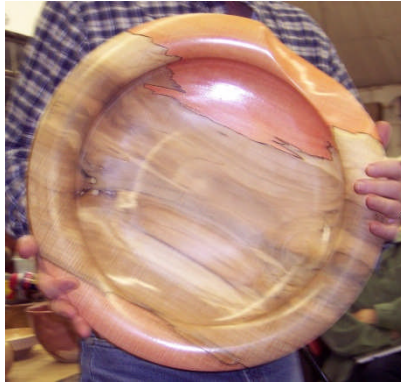
Andy Osborne has this very large spalted Maple bowl which he turned outboard. He then dyed the outside edges with watered down red water based aniline dye before finishing it with four coats of urethane. He enhanced the spalted lines to keep the stain from running. Andy's multi axis pieces
