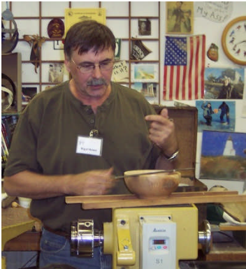
Nigel showed us how to measure the outside depth of a bowl by first measuring the inside as pictured to begin his demo on jamb chucking.
