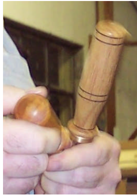
Tim Rix turned some tool handles from Ash and finished them with boiled linseed oil.
