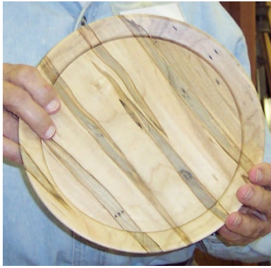
Sidney is holding an ambrosia Maple plate turned flat. The initial finish had a yellow cast to it so he sanded it off and used a lacquer spray for his final finish.
