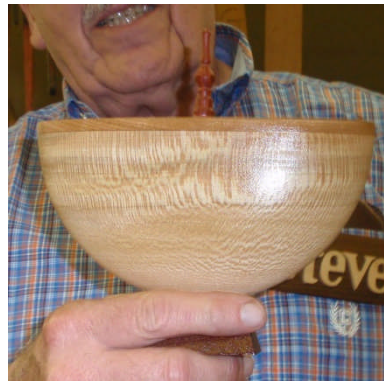
Steve showed us a piece inspired by Alan Carter at the Totally Turning Symposium. It's maple and cherry with a red heart top and mahogany base. He turned a plate and cut it in half and glued it together.
