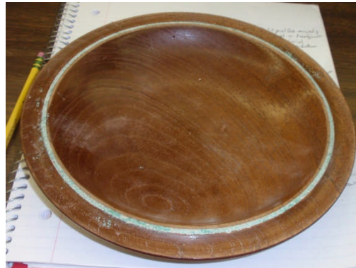
You are looking at the rim of a Cherry bowl with Turquoise dust applied, glued in but not sanded.
