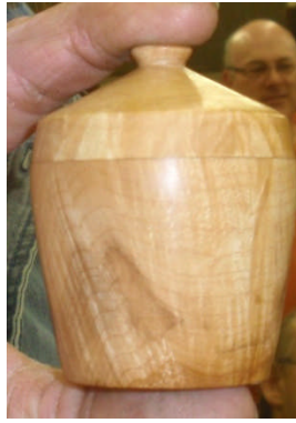
Ian showed a small box turned from California Olive wood. The blank was sold as a bottle stopper but it was too nice not to make it into a box. He said to fit a tight lid you just sand the rim of the box, but to tighten a loose rim, you can put three small drops of medium CA glue on the rim interspersed at equal distances.
