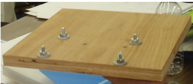
Bob Allen showed a bracket with a track on the bottom you can mount in a vise to save space in your shop. You can mount things like a buffing machine to it for temporary use.
