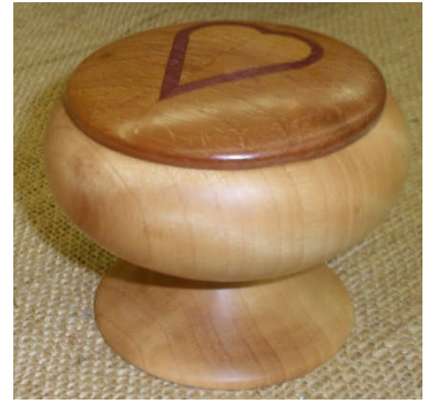
Ian showed a small box turned from California Olive wood. The blank was sold as a bottle stopper but it was too nice not to make it into a box. He said to fit a tight lid you just sand the rim of the box, but to tighten a loose rim, you can put three small drops of medium CA glue on the rim interspersed at equal distances.
