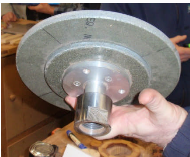
Ian also has a wheel of MDF mounted onto a face plate that he can attach to the headstock on his lathe as an alternate sanding technique.
