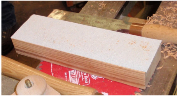
Pictured is the 12" sanding block for sanding each segment to "remove the fuzz".
