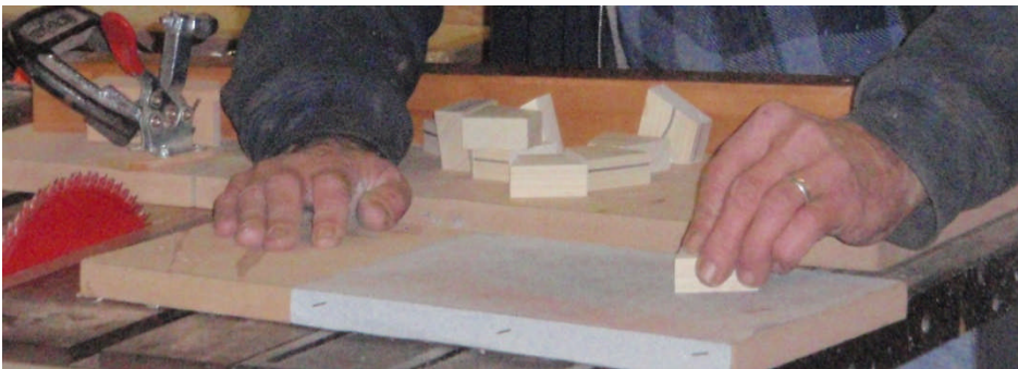
Ian showed us the sanding technique he uses to "knock the fur off each piece". Pictured is a piece of MDF with 60 grit sandpaper glued on. Ian recommends sanding in one direction only and to keep the piece flat to avoid rounding the edges.
