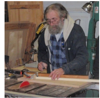
With the sled mounted on his table saw, Ian proceeded to cut out the segments for the first ring
