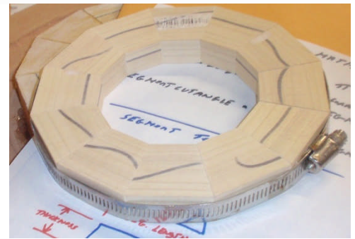
Ring of segments marked all on the same side and held together with a set of radiator hose clamps to check for daylight coming through prior to gluing them together.
