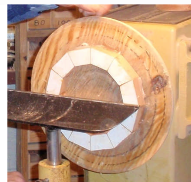
Ian has mounted his glued up ring on the headstock of his lathe to true up the side. This is also an opportunity to adjust the thickness of the ring if necessary.
