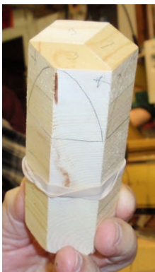
Glued up pieces prior to being cut out on the band saw for a tulip.
