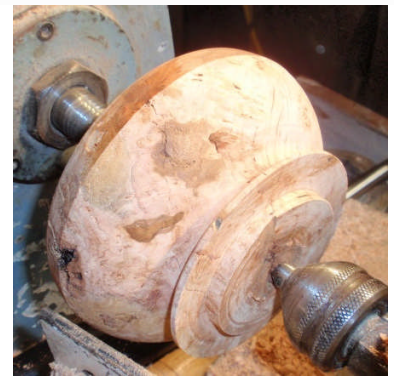
The bottom of the box is shaped
