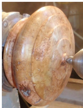
Box now has the lid fitted, formed, sanded and finish applied
