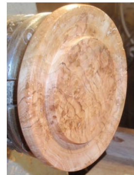
The lid is mounted in the chuck and the under side has a recess shaped into a concave form, then cut around a raised tenon to fit into the box bottom
