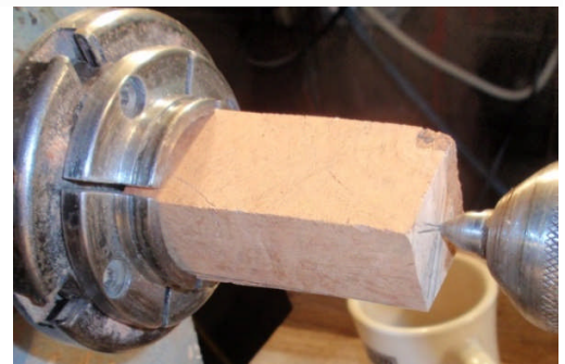
A Nova chuck holds a small piece of Cherry burl that will be used for the stem of the box.
