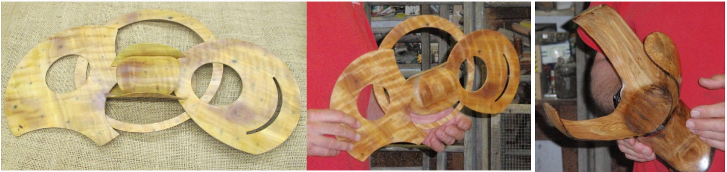
Unassembled pieces turned and bent by Nigel in preparation for constructing his wall hanging. He made it by submerging the pieces in water then taped the curved surfaces to different objects for the different shapes. He had already turned it nice and thin. Nice piece.
