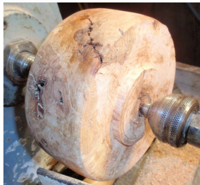
Blank is mounted between centers and a spigot is formed to mount in a chuck
