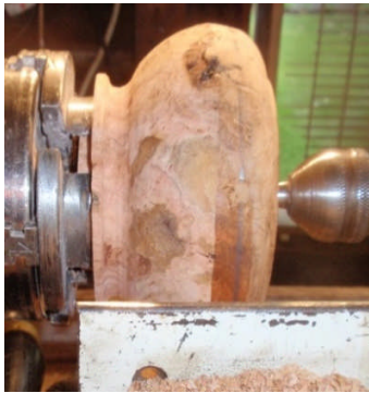
Box is flipped around, mounted in the chuck and marked prior to cutting off the lid
