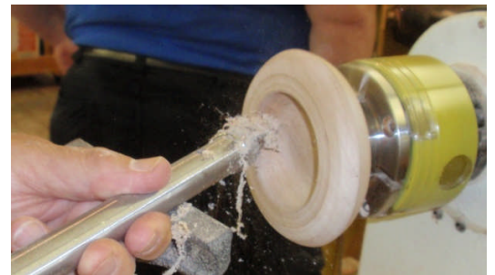
Peter uses a special tool to hollow out the inside.
