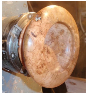
Box has been hollowed out, sanded and had finish applied (Myland's Friction Polish)
