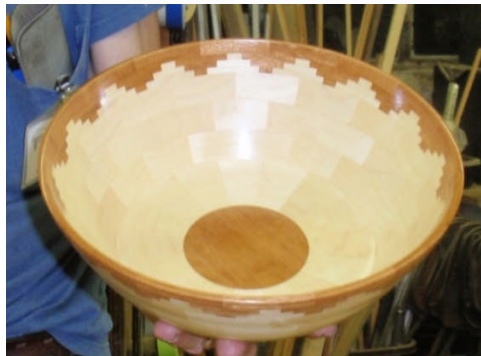
Ian holds a segmented bowl which he said he took about 6 hours altogether to glue up and turn. The woods include Jatoba ( South American Cherry ) for the dark pattern with Maple. The bottom is a stepped plug glued on just two sides to allow for expansion.
