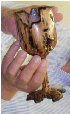
Pictured is a distressed wood goblet turned by Ken Lindgren. He first shaped the outside, sanded it and added a couple of coats of two part epoxy. He used a dentist drill to pick out the bug scat. Next he used a hollowing tool on the bottom. The hard part was carving the stem. For the base Ken used a Dremel tool and a blow torch. The wood is Dedham maple.
