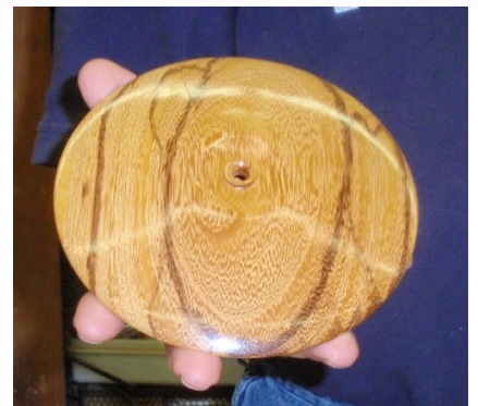
Andy again with a solid block which he cut in half, cleaned out the inside. The key is to get it tight enough and to also match the grain on both halves. It's turned from Marble wood.
