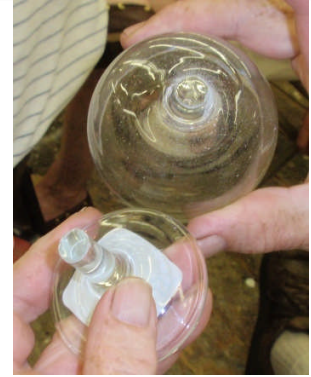
Continue to apply pressure, on a second pass the glass should break cleanly, with no sharp edges.
