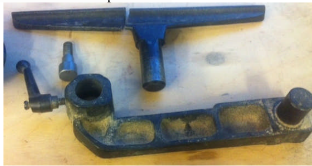
Included with lathe are banjo, tool rest and chuck assembly
