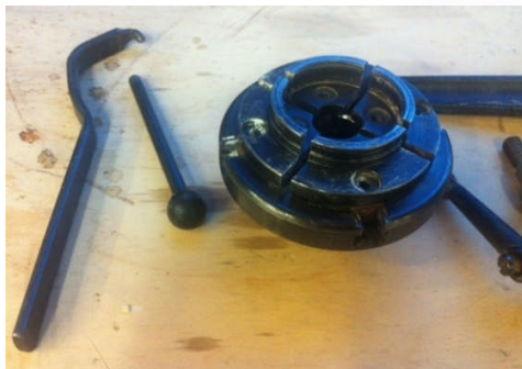
Included with lathe are banjo, tool rest and chuck assembly
