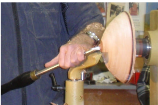
Steve forms a tenon on the base of the blank. Notice the burn mark on the rim from the previous coring made by the cutter.
