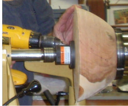
He mounts the blank on lathe and attaches a small faceplate for re-centering if necessary.
