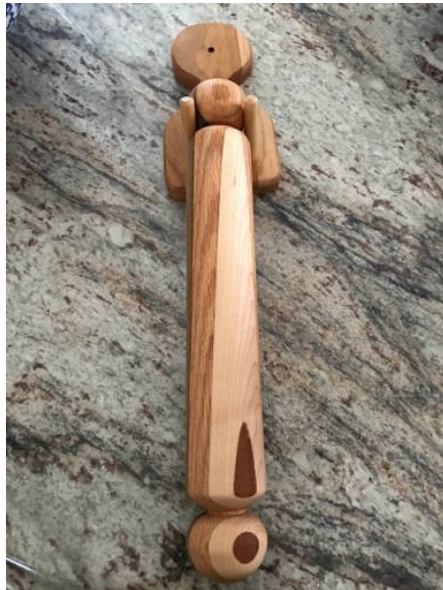
Peter Soltz had a rolling pin turned after glueing up 18 inch scrap wood and cut on a 25 degree angle from a template with a band saw.
