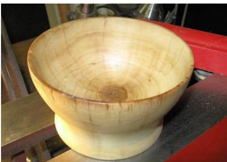
Bob Courchesne turned an aspen bowl with the pith in the center which developed a crack on the lip
