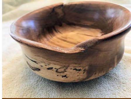
Small bowl turned from apple with a nicked rim. After turning and finishing it with tung oil, the top edge cracked and a piece popped out. By Horace Lukens
