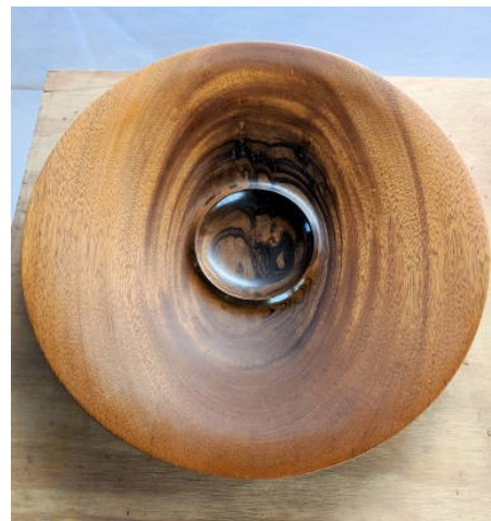
Len also showed us a platter from mahogany 14 1/2" in diameter which has a knot in the middle. Len added a ring in the center for variety as shown. Finished with friction polish and buffed.
