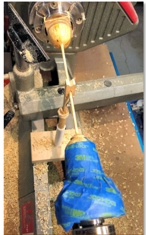
This image shows the thin stemmed goblet mounted on the lathe after the cup was hollowed. Charlie used a steady rest, a clothes pin, to secure it along with the padding he added to hold the base.
