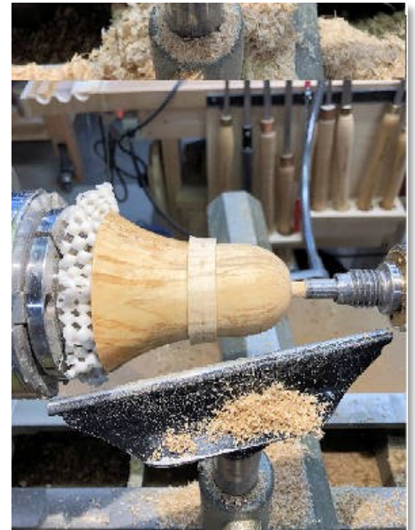
Pictured, Charlie's burl goblet remounted for the removal of the tenon from the flute.
