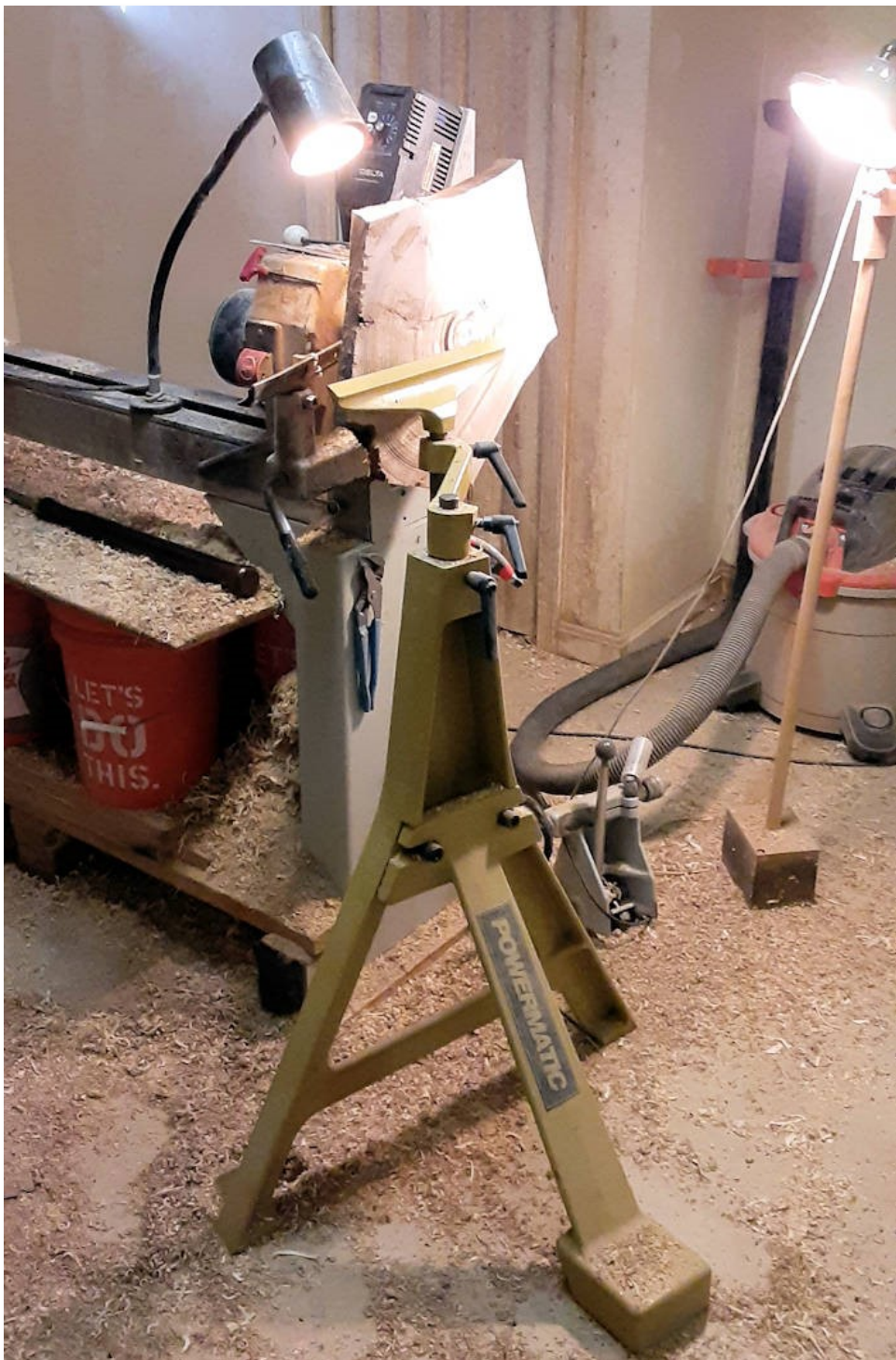
Ken Lindgren showed us his use of the club off-lathe tool rest, positioned to turn a good sized blank. Ken said the tool rest weighs in at about 200 lbs.
