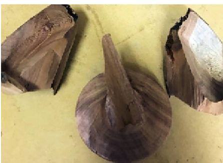
Pictured, was a natural edge bowl that flew off the lathe and broke into three pieces. Oh well sometimes bad things just happen.
