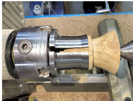
Pictured, is the mounting of the goblet by the tenon formed halfway up the flute with extra long jaws.
