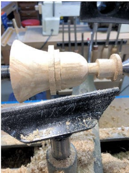
1 of 4 photos taken by Charlie McCarthy of his burl goblet showing different mounting procedures. Here, you can see the tenon formed halfway up the flute.
