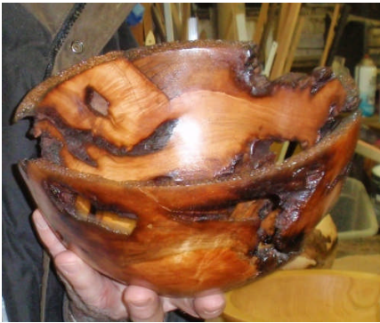
Ken holds a piece of distressed Cherry. He turned the outside, sanded, wrapped it in duct tape then hollowed it out. He decorated the rim with a piercing tool. Next he mixed a tablespoon of Drano with water and painted the outside to give the surface a richer color. Lastly he hit it with a blowtorch.
