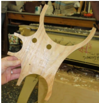
Nigel uses three different sized jaws (2", 4" and 6") and the template shown allows him to determine the tenon size.
