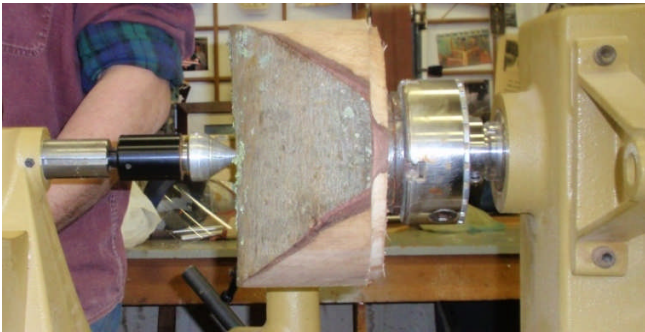
The bowl blank mounted on the lathe. Nigel used a screw chuck in which he predrilled a hole in the center to accommodate screwing the blank into the chuck for support.
