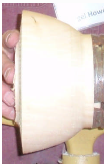
Blank has been turned around and mounted.
