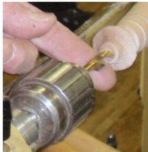
Drilling the handle to accept the guide
