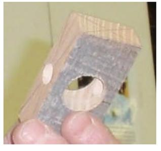
A piece of stock drilled to be turned as a guide
