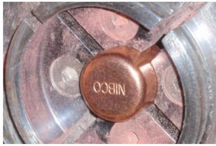
Mounting the copper ferrule prior to drilling it to fit on the handle
