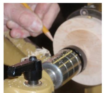
The top mounted in the lathe with the centerline being marked
