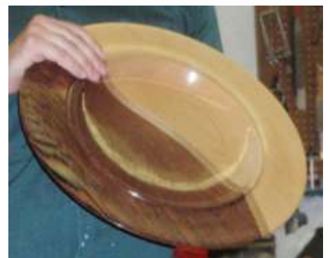
Steve Wiseman holds a platter with veneer bands in the center of Wenge and hard Maple with a true "S" curve. The flush trim is two parallel curves. He then turned a recess and finished with gloss lacquer and hand rubbed it.
