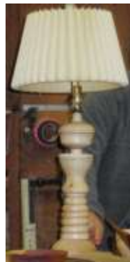
Glenn Shaffer's lamp was turned in four different sections to enable getting the pipe through the inside correctly. He used a burned line decoration on it.
