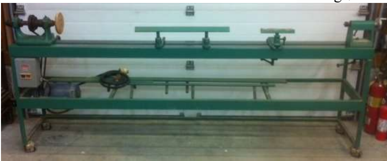
The lathe has a 4" steel frame bed, an 11" swing, and there is 63" between centers. It is powered by a 3 phase 1 1/2 hp. motor with a jack shaft.
