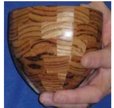
Wayne showed us a segmented piece made from MDF inserted into the middle of two blocks of wood then turned as a bowl, sanded and finished. He then broke the paper glue joint and glued it back together. It has a brush on lacquer finish and wax.
