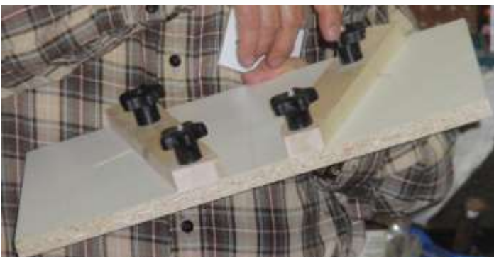
Pablo showed two jigs he made – one for cutting segmented pieces of wood with and a second jig for sanding pieces. He also showed us a segmented vase of light and dark wood with a non-segmented top.
