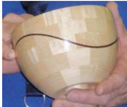
Wayne Miller showed a Birds Eye Maple segmented wave bowl. The wave shaped piece is Wenge which he machined to 1/8 of an inch then soaked it, micro waved it and bent it. He made a special jig to cut the arc.
