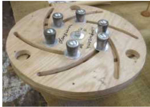
Lenny Mandeville Longworth chuck and depth gauges
