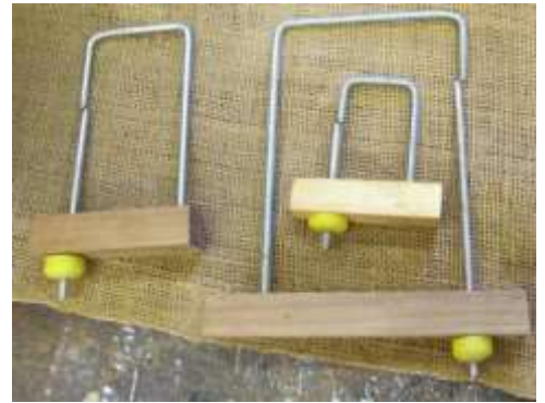
Lenny Mandeville Longworth chuck and depth gauges
