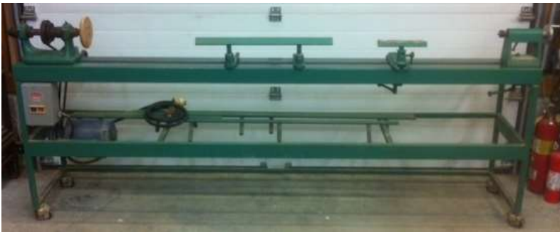
The lathe has a 4" steel frame bed, an 11" swing, and there is 63" between centers. It is powered by a 3 phase 1 1/2 hp. motor with a jack shaft.
