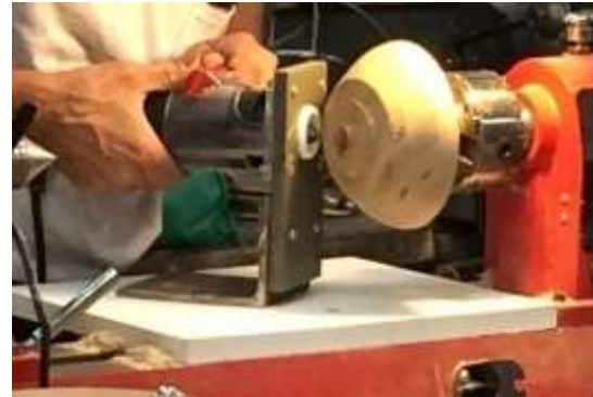
Sliding the router assembly against the blank
