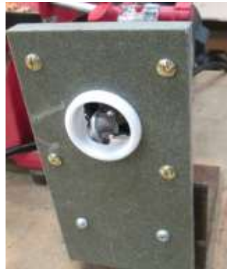
Front view of the router. The router is mounted to a Corian plate which is secured to a Steel Angle iron section.
