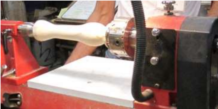
Ian starts with a flat table secured to the lathe bed.
