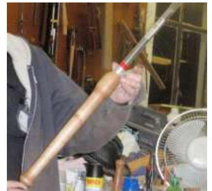
Dan showed us a Thompson Tool bowl gouge with which he turned an aluminum collar. He utilized the leg from a telephone table made of Rock Maple for the handle
