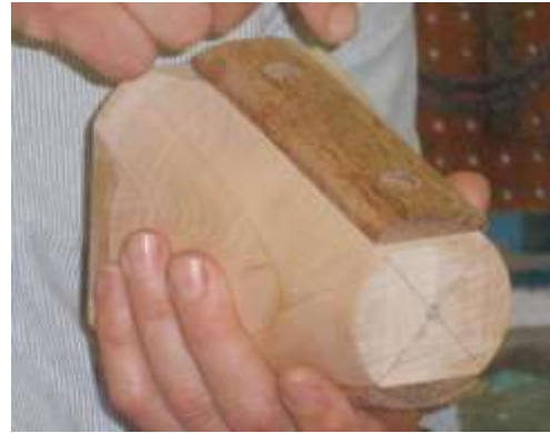
Mike Veno showed us this jig he made to hold two handles for pistol grips for his son's Air Soft game. He used Monkey wood. Since he wanted them to look old, he heated and seared the edges and then applied black shoe polish to the rest of the surface. Grips are screwed on to the jig recessed screws
