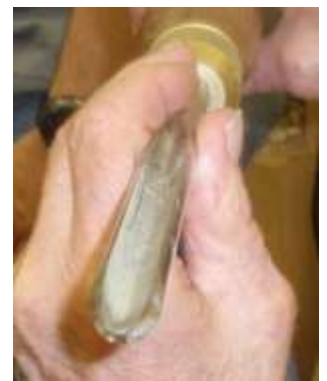
Three views of Nigel's 5/8th inch bowl gouge with his modified Ellsworth grind. He puts a second bevel toward the end of the tip for cutting around the inside curve at the bottom of the inside of the bowl. It prevents marking the curve from the edge at the end of the bevel on the outside of the tool as you take it around the bend inside.
