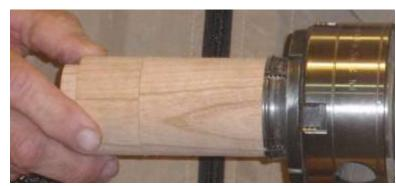
The box is mounted so that the bottom can be hollowed.
