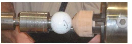
Steve uses a golf ball mounted on a live center on the tailstock to hold the lid onto the box
