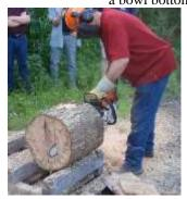
Nigel demonstrates how he cuts off each side of the tree to make it ready to mount on the lathe.
