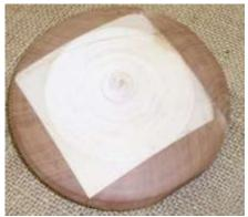
Wally made a larger tenon to hold his goblets by glueing waste wood around the outside of the base. Wood is sugar maple from a fallen tree in Jeff's front yard.
