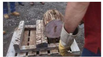
Nigel brought along a converted pallet he uses to position logs for cutting.
