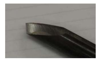
Using the skew on the grinding wheel will produce a hollow grind. Steve said that he hones two tools; the skew and the parting tool. Steve said he likes the hollow grind on the skew. He uses a diamond card on each side.
