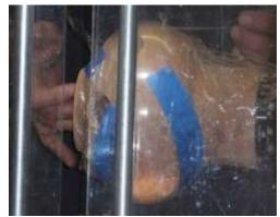
He uses cellophane wrap to keep his hollowform from drying out between turning sessions as is pictured here. Blue tape holds it in place
