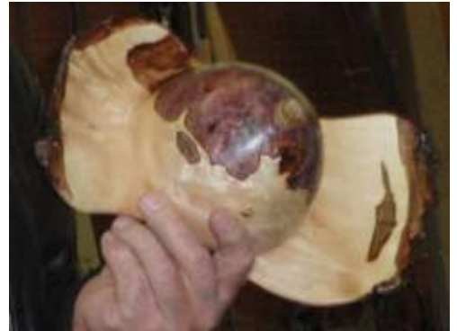
Ken holds one of many small burl bowls with a bark rim which he then cut away the sides. It has a dyed base which is actually one of three he made for comparison purposes. He outlined the edge of the burl with a piercing tool which allowed for a thin indented line before coloring some of the wood. It has a wipe on poly finish on the bowl while the base has a bar top finish of epoxy. Ken said that Angelo Iafrate had once told him, "If you don't care how long it takes to make it, it is amazing how nice it becomes."
