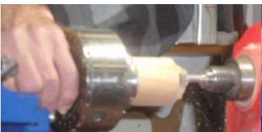
Cutting the outside threads on the top for the lid.
