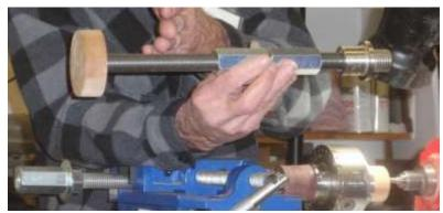
Here is the jig with the collett chuck at the end ready to accept the larger chuck.
