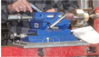
Pictured is the slide Ian purchased from Harbor Freight for around \$60. It holds the jig (from photo #2) which has been fitted with a Purpleheart adapter/ spacer for the chuck. It is positioned close to the headstock with the cutter engaged in cutting the inside thread of the lid.
