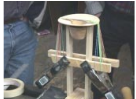
Hat is set inverted in fixture and rubber bands are used to form brim contour
