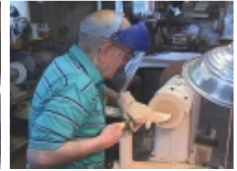
Wally and Sidney are bent on mounting faceplate to fit Sid's piece to Oneway for turning jam chuck
