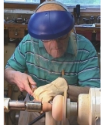
Bowl mounted to the jam chuck and bottom faced off to accept addition to bottom of bowl.
