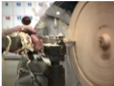
The McNaughton Systems tool is aligned dead center and cuts are made clearing chips often. Wally worries.
