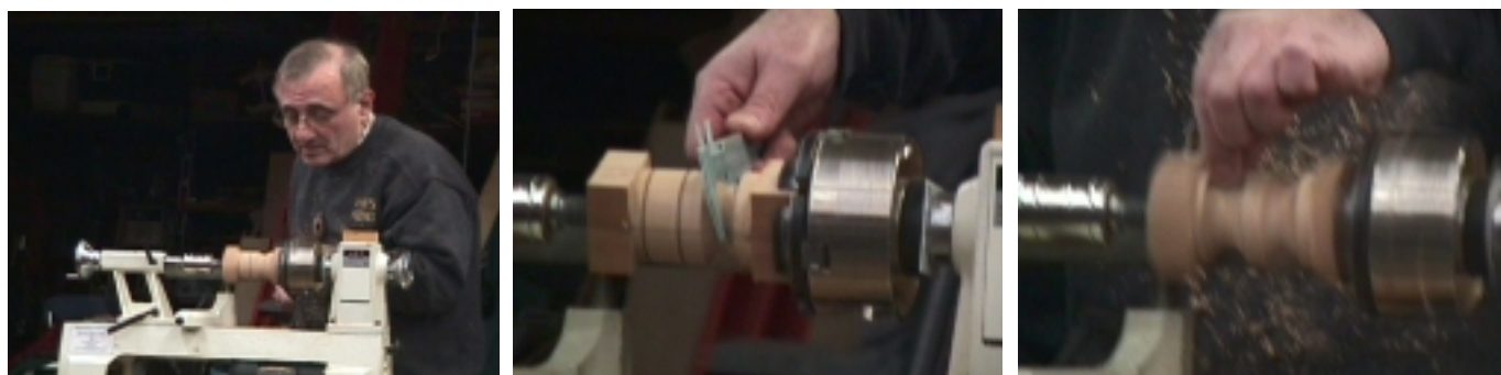
The grooves which will become round holes are turned and measured with calipers and Bob's finger, an available radius instrument. I wouldn't say he's cheap, just frugal, and he does have eight of them, Now!
