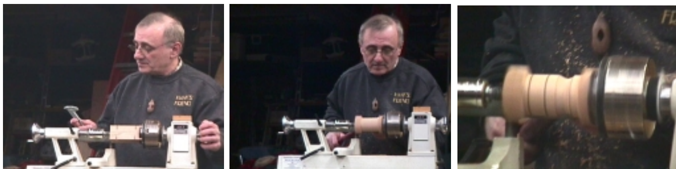
Glued up blank with paper joints is mounted on lathe and calipers set to turn inside details. Bob now uses a One Way cup live center and four jaw chuck to eliminate initial gluing.
