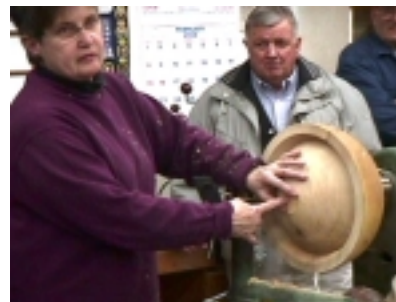
When 1" to 2" diameter is left to cut tap the edge of the core to break it loose. Prepare base for next coring.
