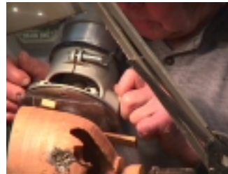
Rout bow tie cutout with straight or spiral bit and collar. Clean up corners and glue in contrasting bow tie.
