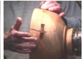
Rout bow tie cutout with straight or spiral bit and collar. Clean up corners and glue in contrasting bow tie.
