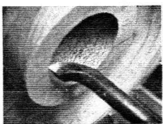
Precision boring a crankshaft hole and crankcase center section
