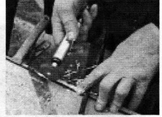
Carefully grind soldered area to blade thickness
