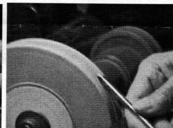
Turning handle for a round skew - grinding the "screwdriver" shape on HSS shaft and final skew angle as shown ( See Bob's article "Making a Skew" in American Woodturner Summer 2001 page 37 )
