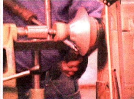
As more pressure is applied to the material it slowly flows to the form
