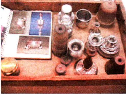
Album of Bob's work with forms and chucks use in metal spinning. He worked at Reed & Barton
