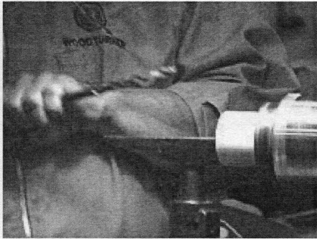
Getting started with the plunging of a drill into the mounted blank
