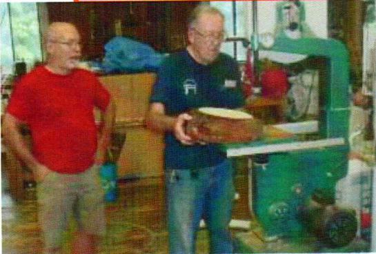
Prior to turning, Matt watches as Steve uses a cardboard pattern to cut out a round blank from his piece of Cherry.
