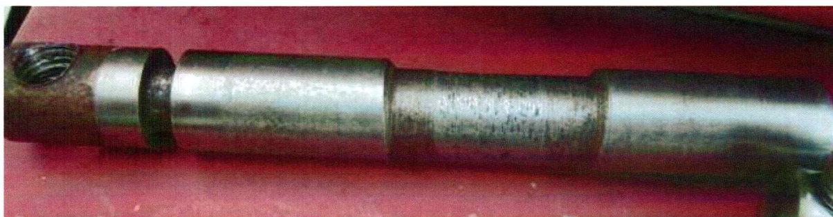
Old worn shaft
