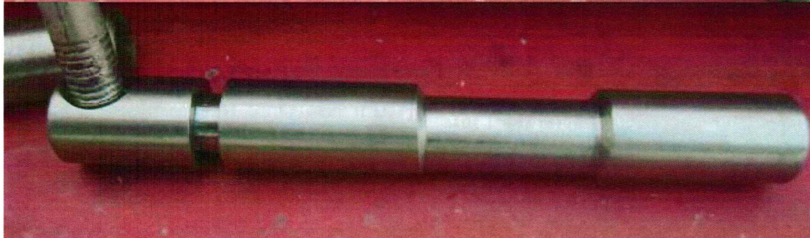
Replacement shaft - courtesy of Bob Monaghan who took his metal lathe and turned the replacement.
