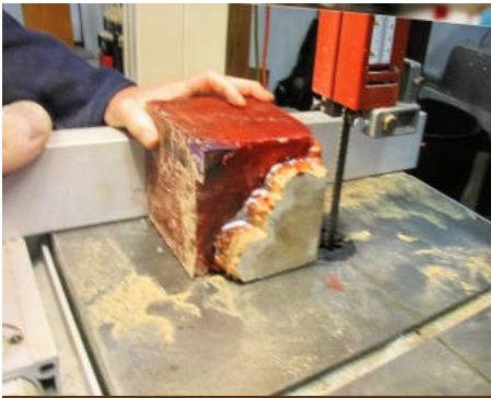
The resin block has been removed from the pressure pot and its' mold
