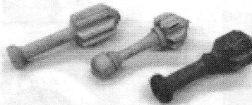
Roger cut grooves on lemon juicers on table saw before turning
