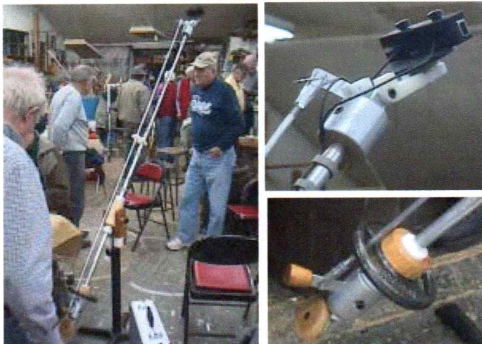
Don Diedrich fabricated a dual camera boom for viewing and recording our demonstrations. Note counterbalance weight!
