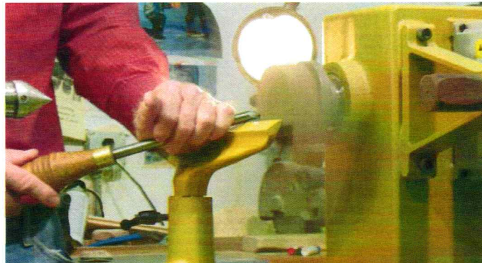
Positioning the gouge for cutting
