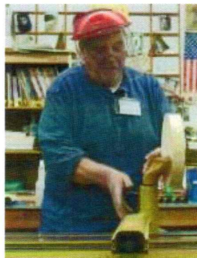
It has been drilled and turned with a recess cut into the opposite side which Lenny is mounting in the chuck.
