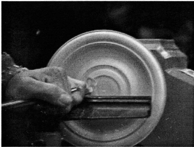
1. Hollowing bowl after shaping rim and finishing bottom so he doesn't have to reverse chuck
