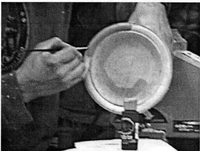
3. A gloss lacquer coating is applied around rim prior to painting with low cost colored acrylic paint
