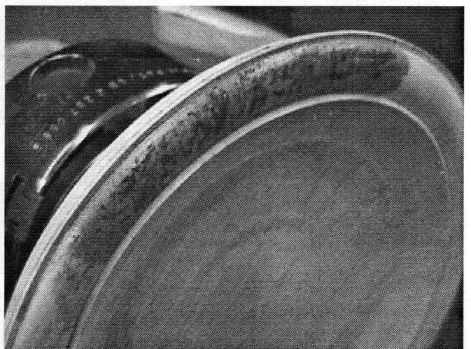
6. Final finish is 2 coats lacquer and wax. Shown is ultramarine blue. Gold stipple makes a nice effect
