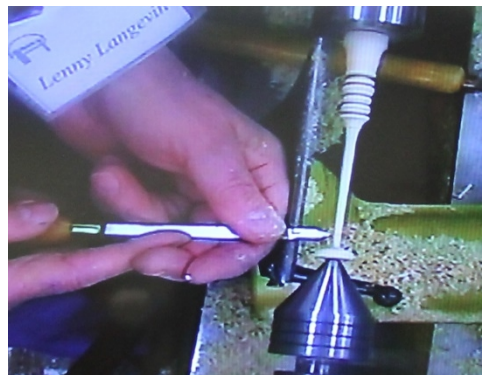
Len is ready to part the front of the pin from the tailstock.
