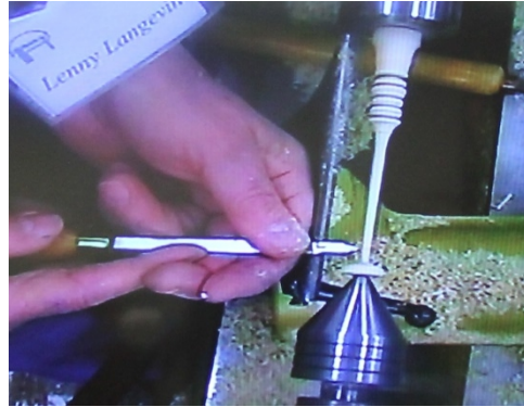
Lenny focuses on the cone part from the shaft up to the decorative part of the pin.
