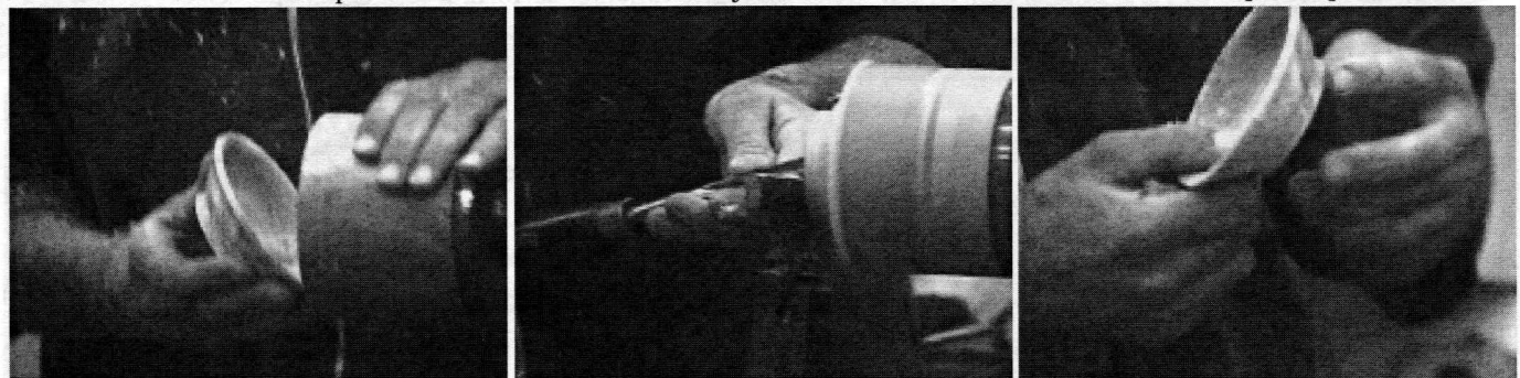
Jam chuck is turned without a taper to fit bowl. T shirt material used for snug fit. Taped in place with masking tape. Bottom turned
