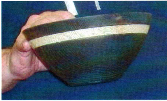
Andy showed two bowls. A woman in Concord wanted some pieces turned to use as gifts. He cores these two pieces. The one on the left was bleached the one on the right was dyed. He finished them using a water base urethane.
