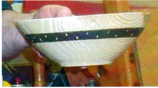
Andy showed two bowls. A woman in Concord wanted some pieces turned to use as gifts. He cores these two pieces. The one on the left was bleached the one on the right was dyed. He finished them using a water base urethane.
