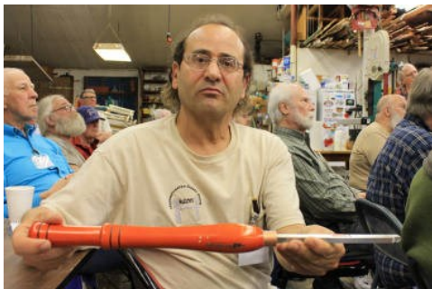
Glenn holds Steve's radius tool. The wheel at the end is both a small surface presented to the resin for light cuts and has a 360 degree wheel which is a long lasting sharp cutting edge.
