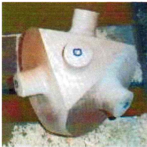
The completed Octahedron before carving off the tenons. Michael said leaving the tenons allows the work to be held in the jam chuck.
