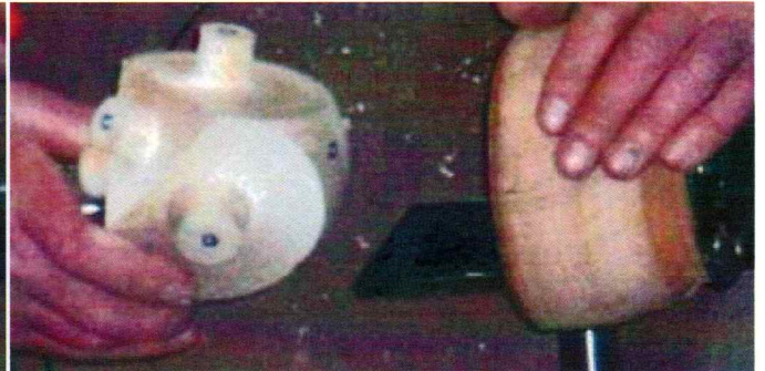
Michael positions the sphere in the jam chuck after marking off the 8 axis points with a compass and turning two of them.
