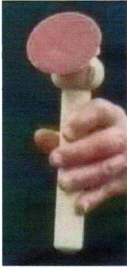
Lenny Mandeville - made a manual sander using a flanged bearing purchased from McMaster-Carr
