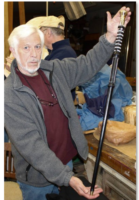
Full view of Wally's Victorian lady's walking stick. Ken Whiting did the vertical slits for beads and also five equally spaced diameters for Wally's friend, Chris Brenner to apply the jewels. Stick is turned from maple and dyed black.
