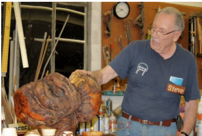
Steve showed us a piece of Gateway Club wood - sugar maple which has a nice color and texture. He mounted it on a faceplate and turned it. Parts of it have a glass like finish. It is mounted on a lazy susan. The inside was hand carved to hollow it.
