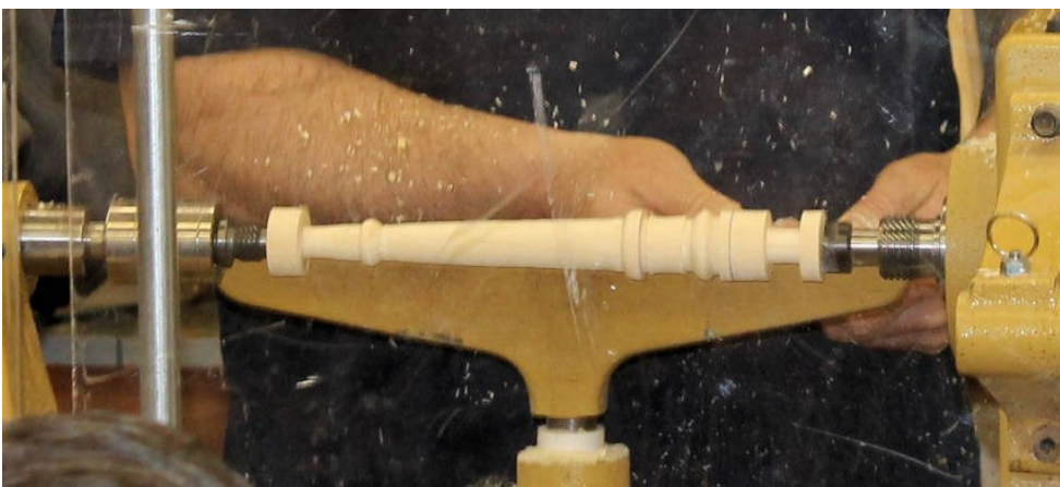
Bob has nearly completed turning the leg now.
