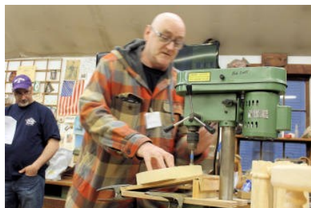
Fred has the jig in place on the drill press with the stool seat positioned on it for the proper angle prior to drilling
