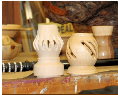
Pictured is a closeup of Bill's two hollow forms showing some creative vertical and twist decoration. Bill measured eight different sides on the lathe in the chuck then marked off spacing and used a hacksaw to remove material. He finished smoothing the openings with a file.
