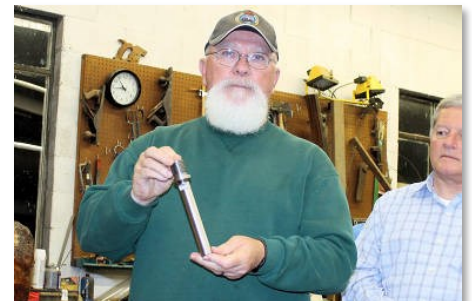
Charlie showed us this one inch metal post that Bob Monaghan made for him to fit into his lathe's tool rest
